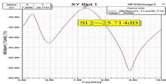
Fig10. Mutual Coupling S_{12} = -25.714\text{ dB}
