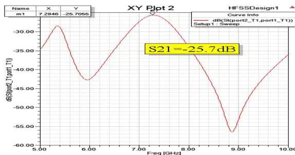
Fig11. Mutual Coupling S_{12} = -25.7\text{ dB}
