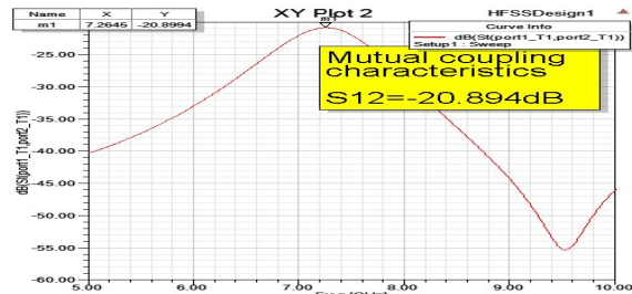
Fig 5. Mutual Coupling S12 = -20.894 dB
